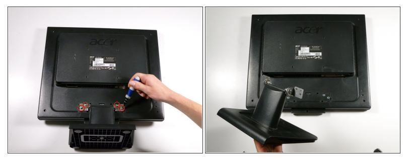
• Remove the four 12.1 mm Phillips #2 screws that hold the stand to the monitor.
