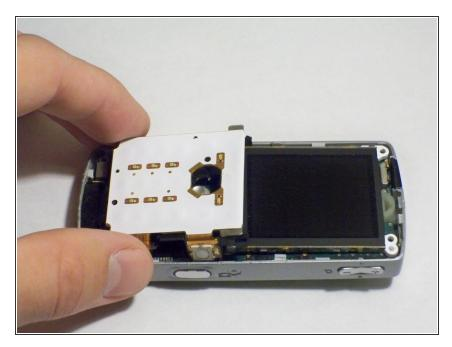
Gently lift the base of the keypad to remove it.
