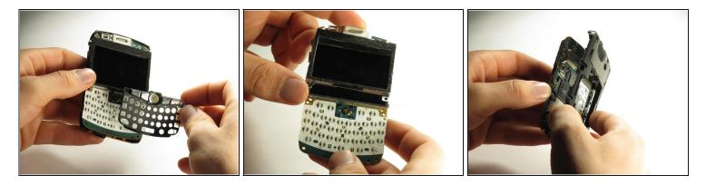
• When all four screws are removed, the keyboard frame, screen housing, screen, and back casing can be separated.
