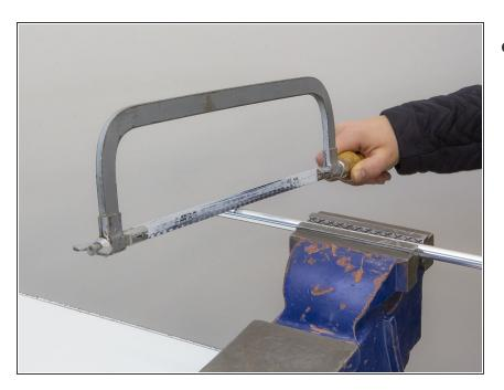
• Put the pole segment into a vice and saw it off at the correct length.
