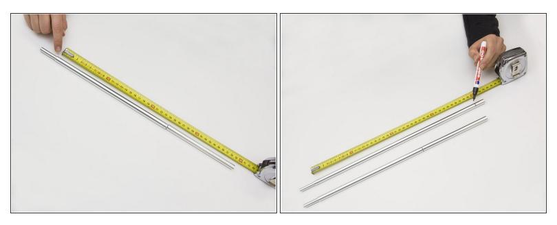
• Transfer the length of the broken segment to the new segment. Start measuring after the tapered end, and mark the length with a marker.
