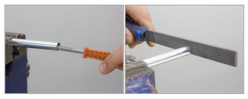
• File off any sharp ends using the round file on the inside and the flat file for the outer edges.
