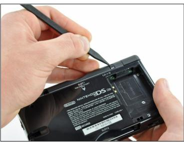
Use the tip of a spudger to pry both rubber feet off the DS Lite.
