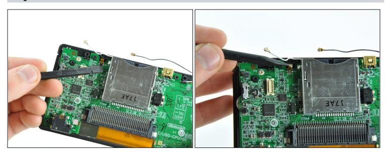
• Use your fingernail or the edge of a spudger to carefully flip up the touchscreen ribbon cable retaining flap.
