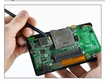
Use the flat edge of a spudger to pry the Wi-Fi antenna connector straight up from its socket on the Wi-Fi board.
