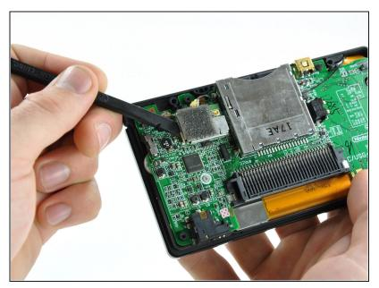
Use the flat edge of a spudger to pry the Wi-Fi board connector straight up from its socket on the motherboard.
