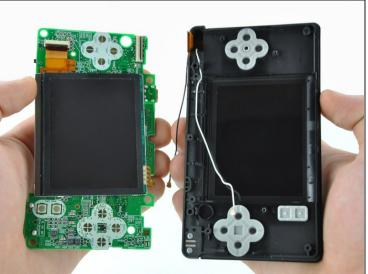
• Use your fingernail or the flat edge of a spudger to carefully flip up the upper LCD ribbon cable retaining flap.
