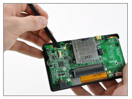
Use the flat edge of a spudger to pry the microphone connector straight up from its socket on the motherboard.
