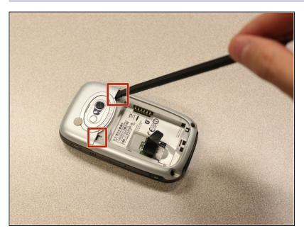
Insert the flat end of the spudger into the two notches on the back of the camera cover and pry them up.
