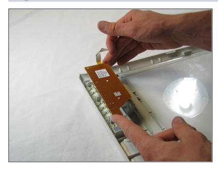
• Using both hands, carefully lift the control panel circuit board from the top panel of the printer.
