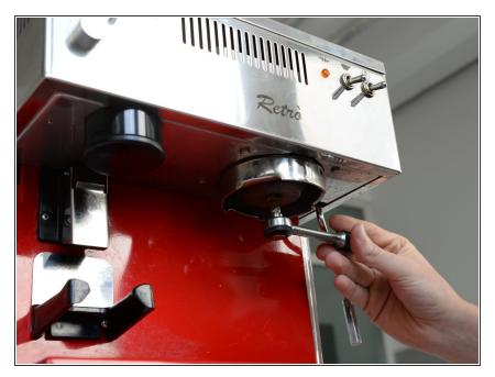
• Remove the flat head screw in the center of the filter hodler.
