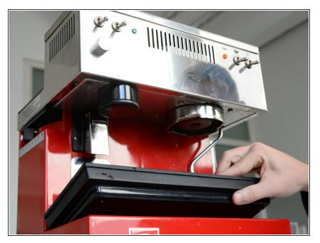
Remove the black tray for an easier disassembly
