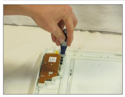
Reattach the plastic piece which holds the scanner glass down and the 2.74 mm Torx screw.
