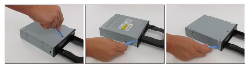
• Push in black tabs on left, right and bottom of outer chassis to unhook faceplate.
