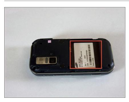
Remove the battery from the phone by using your plastic opening tool to find a gap at any edge of the battery and lifting the battery up.
