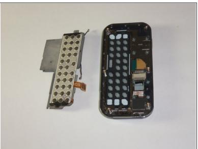
The keyboard chip is located on top of the device. Pry the keyboard off of the case with the plastic opening tool.
