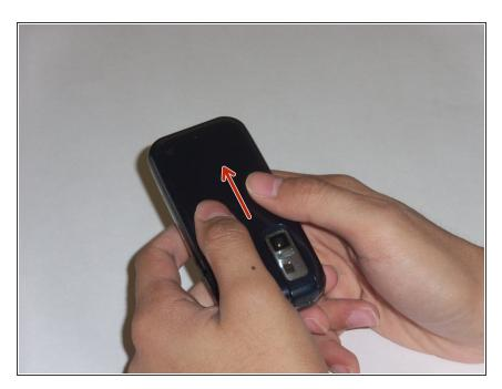
Using your thumb, press down and slide the back cover away from the camera.
