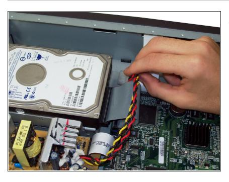
Remove the red, yellow, and black cable connecting the power supply to the hard drive.
