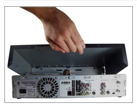
• Lift the cover up and off the device.
