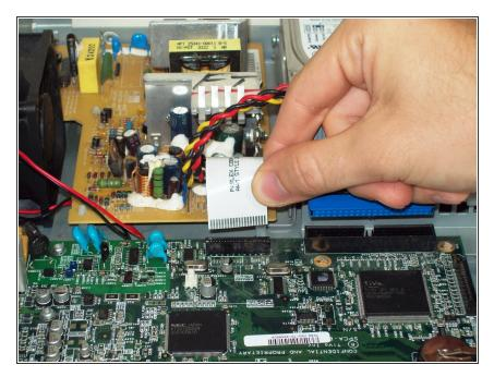
Remove the belt connecting the power supply to the motherboard by pulling it out.
