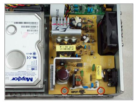
Remove the two 0.31 inch T-9 screws from the power supply.
