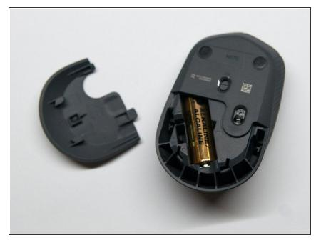
Switch off the mouse and slide out the bottom cover. This is where all the necessary clips can be accessed.
