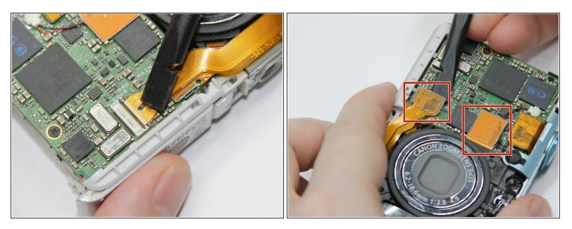
• Use the spudger to lift the tab on the **Zero Insertion Force** (ZIF) connector located at the bottom of the motherboard.
