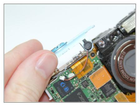
• Lift off the mechanical shutter button assembly.
