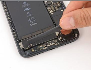
• Use the flat end of a spudger to disconnect the Taptic Engine connector from its socket on the logic board.
