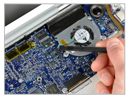
Disconnect the right fan cable from the logic board by placing a spudger beneath the cable and lifting up. Be sure to lift up on the right side as shown.
