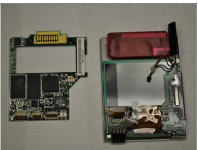
Now that both ribbons and the wire are disconeccted, you can apply a downward pressure to the battery. You will have to carefully rotate the frame so that the battery can go through.
