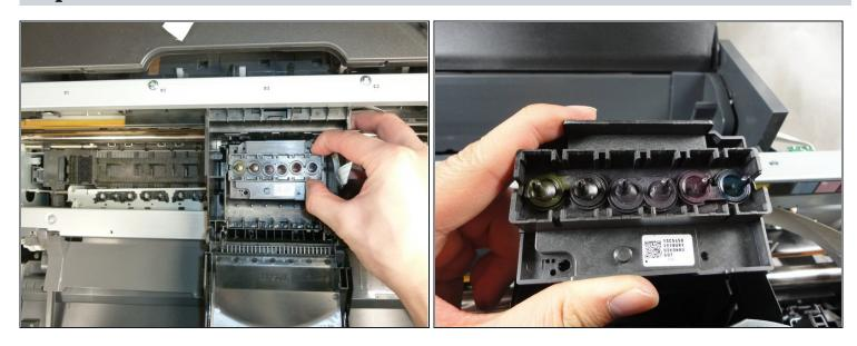
• Remove the printhead from the carriage unit by lifting it up vertically.
