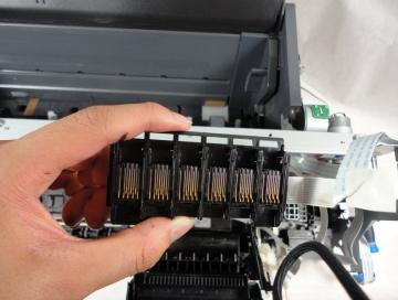
• Lift CSIC assembly up and out of the Carriage Unit.
