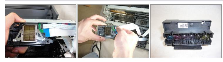
• Disconnect the two ribbon cables on the back of the printhead.
