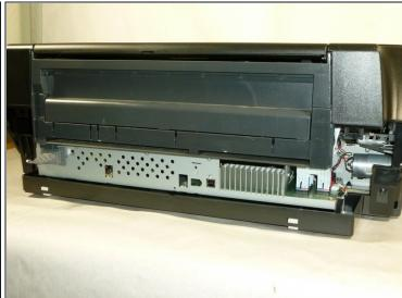
• Remove the rear housing by pulling it backwards.
