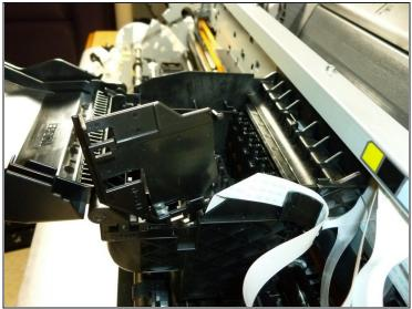
Slide the cover upward and rotate it around the hinge by 90°.
