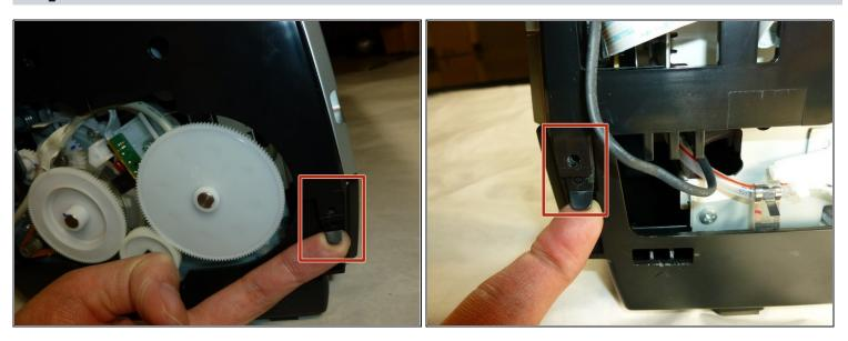
• Detach the tabs from the pins on each side by pulling it outwards.
