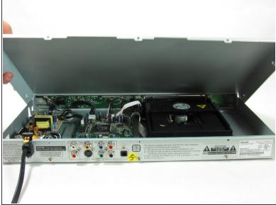
Lift the top panel from the back and remove. It should come off without being forced. There is a lip
