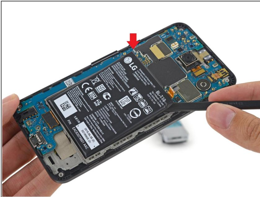
**⚠** ESD or Electro-Static Discharge can damage sensitive circuitry so do not touch anything on circuit board, such as connectors and resistors, with your bare hands!
