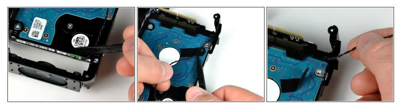
• Flip the frame and then rotate it 180 degrees so that the speakers are facing you.
