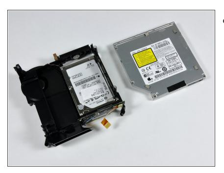
• The SuperDrive should now be removed from the internal frame.
