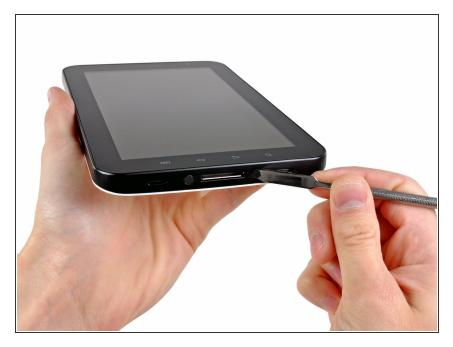
Use the flat end of a metal spudger to pry the two plastic tabs near the dock connector off the rear case.
