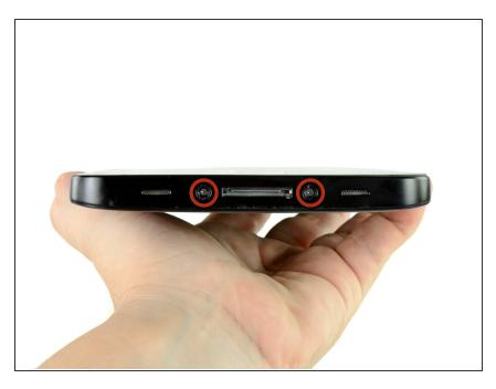
Remove the two 4.1 mm Tri-Wing screws near the adjacent edges of the dock connector.
