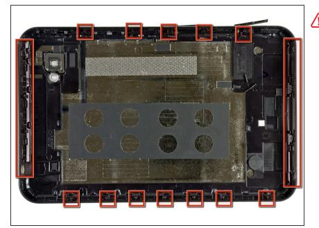
The following steps will require you to disengage several clips (highlighted in red) around the perimeter of the rear case. The clips are delicate and fragile; proceed with caution.
