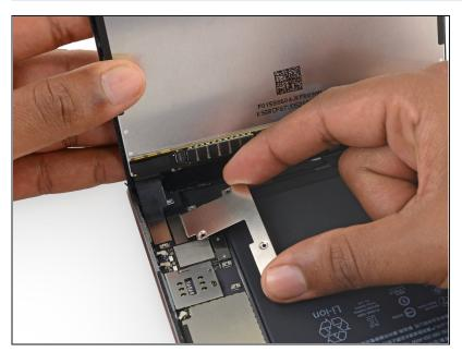
• Remove the battery/display cable bracket.
