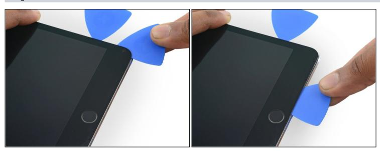
• Slide the pick from the bottom right corner along the lower edge of the device. Stop about half an inch shy of the home button.
