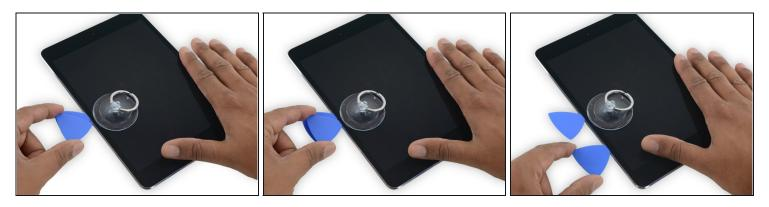
• Insert a second opening pick alongside the first and slide the pick down along the edge of the iPad, releasing the adhesive as you go.
