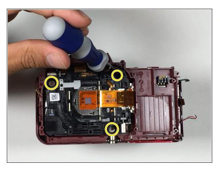
Remove the three 1.5 mm Phillips #1 screws connected to the lens assembly.
