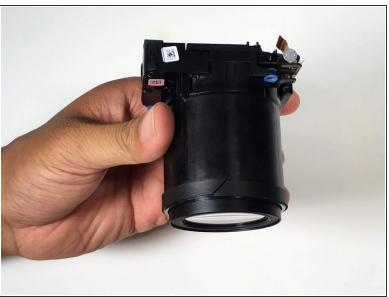
Pull the lens assembly from main body of the camera, using a spudger to pry if necessary.
