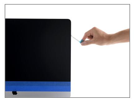
Repeat the previous two steps to remove the protective film from all the remaining adhesive strip pairs (labeled 2, 3, and 5).
