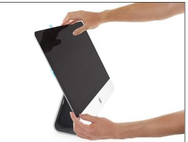
• Gently lay the display in place over the iMac, and align it carefully.
