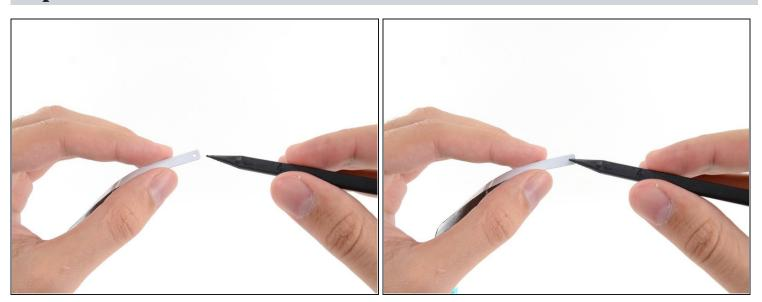
Insert the tip of a spudger into the hole at the end of the strip from the side that still has a backing on it.
