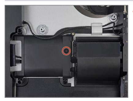
Remove the 7.3 mm T8 Torx screw securing the hard drive tray to the rear enclosure.
