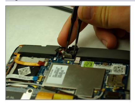
Use the <u>tweezers</u> to pry the camera assembly away from the motherboard.
