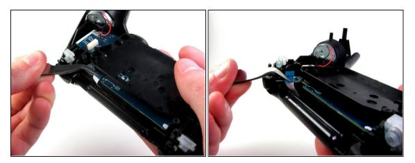
• Gently detach the touchpad ribbon connected to the motherboard using the blunt forceps. The touchpad ribbon is connected to the motherboard by a connector that flips to tighten and loosen. During reassembly, to reattach the ribbon, the plastic tray will need to be gently removed from the motherboard and the flip-lock flipped up.
