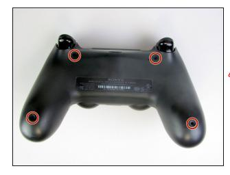
• Using the Phillips #00 Screwdriver, remove the four 6.0 mm screws securing the rear cover to the controller.
