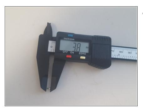
S3, S4, S5 screws are 3.8mm, an extra 0.6mm over the S6 and S7 series.
