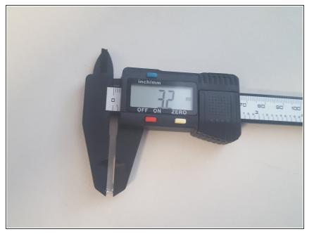
3.2mm S6 / S6 Edge & S7 series screws are 3.2mm.
