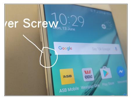
Using 3.8mm screw around edges S6 / S7 Edge will cause damage to the LCD as per photo. Only ever use 3.2mm phillips head screws on S6 and S7 screen replacements.
