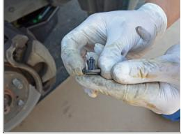
Replace the three push retainers by first inserting them into their respective holes with the inner pin pried up. Push the pin into place to secure each retainer.
