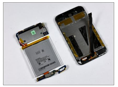
The logic board and battery can now be fully separated from the rest of the iPod.
