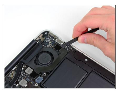
Use the flat end of a spudger to pry the I/O board cable up from its socket on the I/O board.
