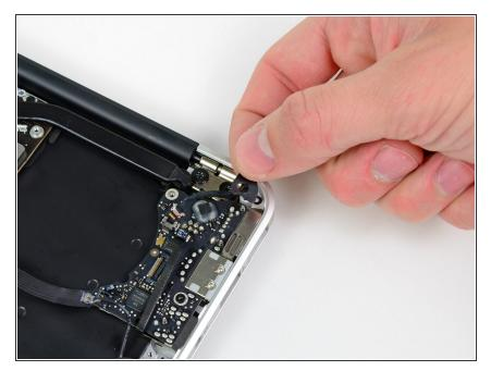
Remove the small rubber gasket from the corner of the upper case nearest the I/O board.
