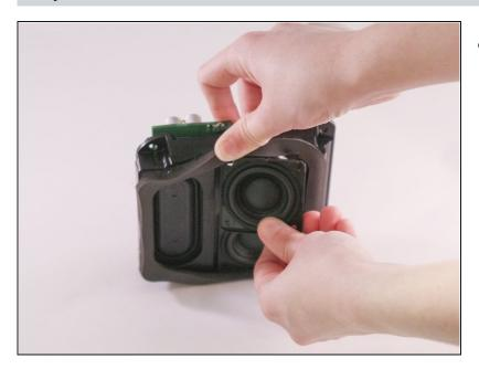
• Push the speaker through the front of the inner assembly.
