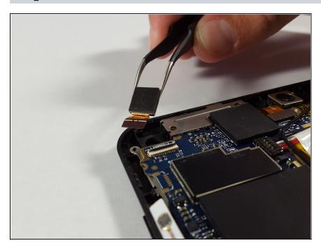
• Remove the front facing camera with tweezers.
