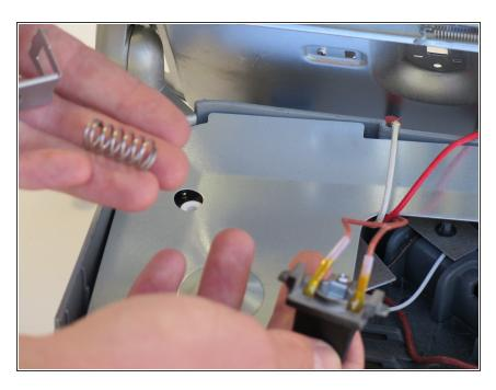
Pull out the spring, and insert the replacement spring making sure it is correctly aligned.
