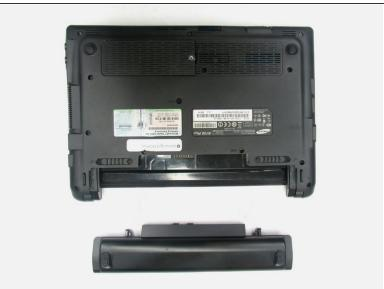
While holding the left and right hand switches in the "unlocked" position, push the battery away from the computer.
