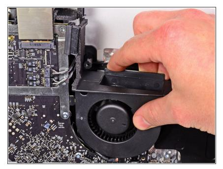
Pull the optical drive fan off the pins attached to the outer case.
