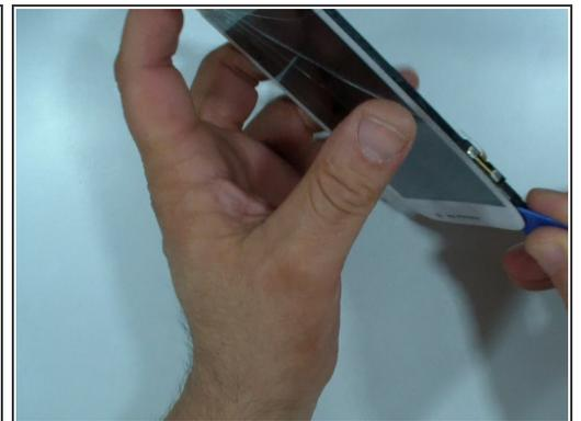
**⚠** At the bottom side, under the touch screen glass is the menu buttons flex cable. Be careful for it when you separating the glass from the frame.
