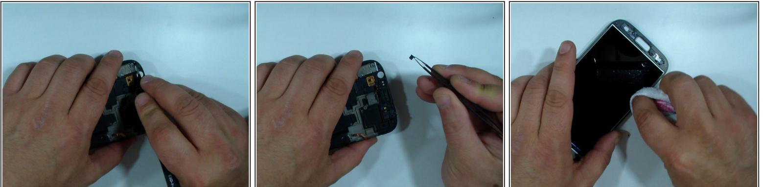
**!** There is a small plate in the touch screen flex cable slot. Remove it to allow the flex cable of the new touch screen to pass.
