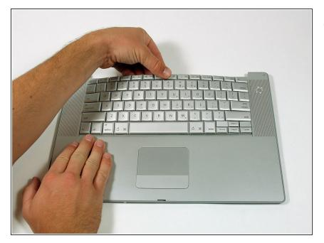
Maintaining your hold on the keyboard, lay the casing flat and gently bow the keyboard until the two tabs on either side of the keyboard come free.
