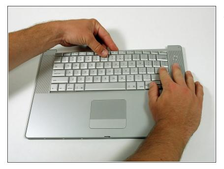
To replace the keyboard, first slide the bottom tabs into the upper case. Then bow the keyboard out and first slide the tabs in on the right side of the keyboard, then slide in the tabs on the left side.
