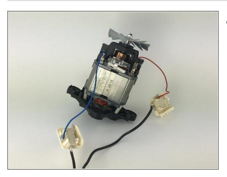
Remove the motor and replace it.
