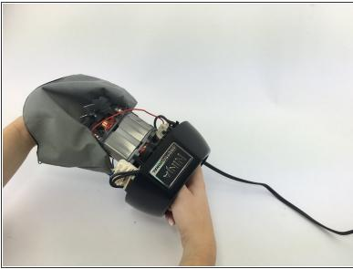
Untwist the small rubber connector to detach the plastic from the motor.
