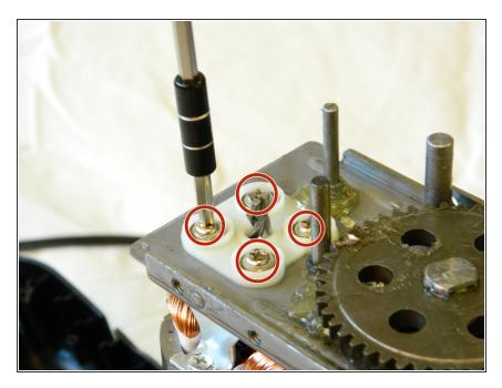
Remove the four 18mm PH2 screws holding the motor to the main shredder assembly.
