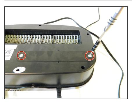
Remove the two 10mm PH1 screws holding the small black panel in place.
