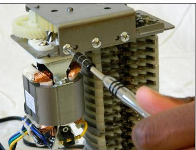
Remove the five 8mm PH2 screws from the bracket holding the gears in place.
