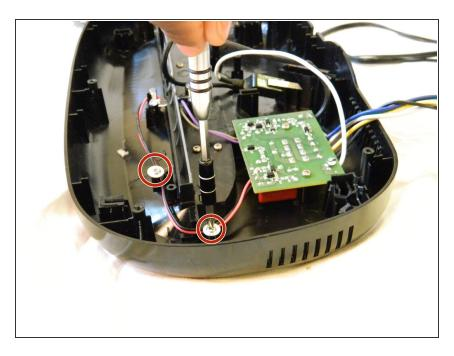
Remove the two 8mm PH1 screws holding the IR sensor wire in place.
