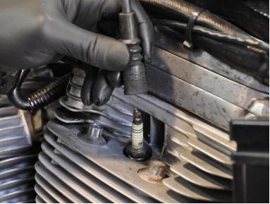
Carefully remove the spark plug wire. Do not pull on just the wire, squeeze the spark plug boot, and pull it together with the wire.
