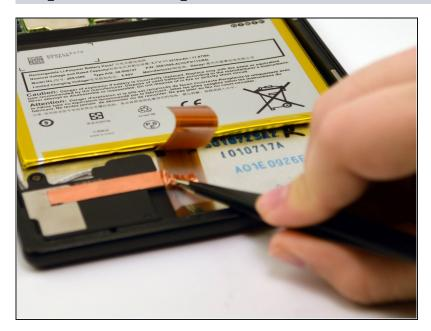
Using tweezers, carefully lift the copper strip from the right side of the speaker.
