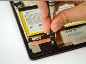
• Remove the two screws located on the top left and bottom right of the speaker using a T4 screwdriver.
