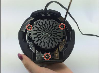
Turn the blender over and unscrew the three 14 mm screws holding the slotted base in place.
