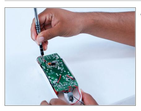
Remove the two 10 mm screws using the 1/4" driver and a J1 Phillips screw head.
