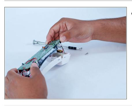
Carefully move the motherboard up to remove it.
