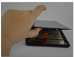
• To remove the screen from the device, use <u>tweezers</u> to gently pull the orange cable from its connection to the screen.
