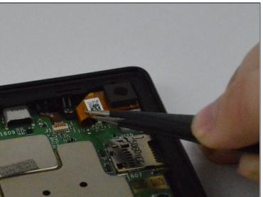
• Pop the camera out of the rear-facing camera casing by carefully pulling the orange cable with the <u>tweezers</u>.
