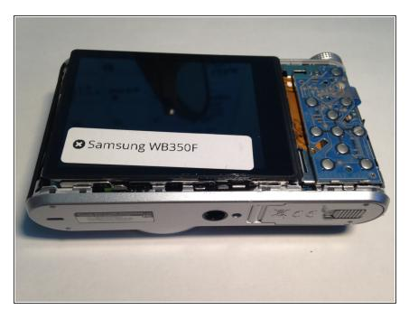
Remove the plastic casing, exposing the inner workings of the camera.
