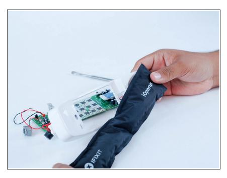
Use the iFixit iOpener to warm the adhesive from the front of the phone, in order to remove the speaker from the face plate safely.
