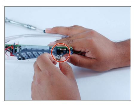
Remove the speaker volume switch before trying to separate the keypad
