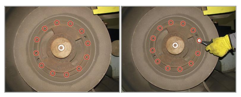
• Remove the twelve bolts securing the grindstone using a ratchet with a 5/16 Hex bit.
