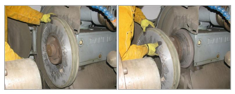
Carefully remove the grindstone itself from the spindle, making sure to support it from the top and inner ring.
