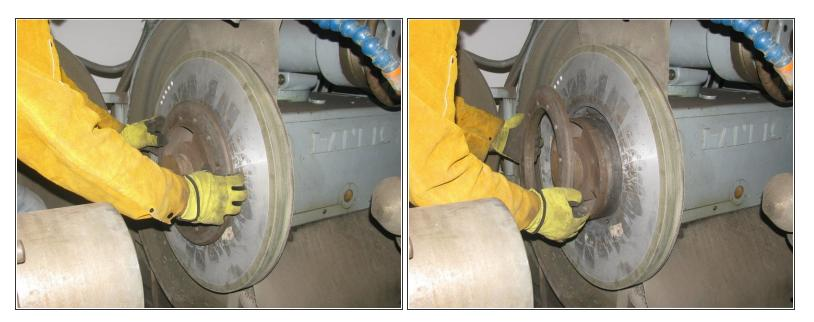
• Gently remove the steel hub from the grindstone spindle.
