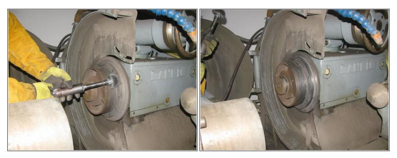
• Softly sand the hub with 600-grit sandpaper or a wire brush to remove any surface rust.
