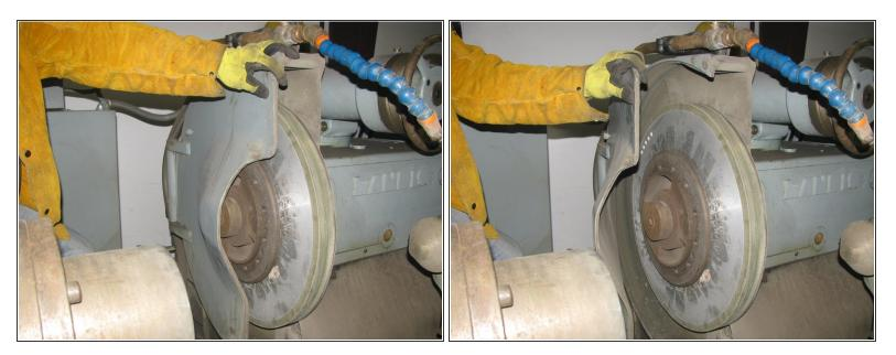
• Pull the access panel outward to expose the grindstone.
