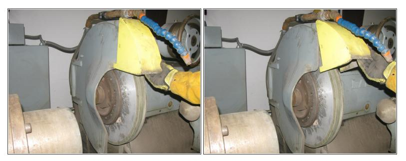
• Lift the yellow guard up to unlock the grindstone access panel.
